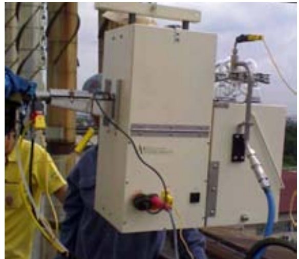
Measuring air quality at the stack of a spirits production site
